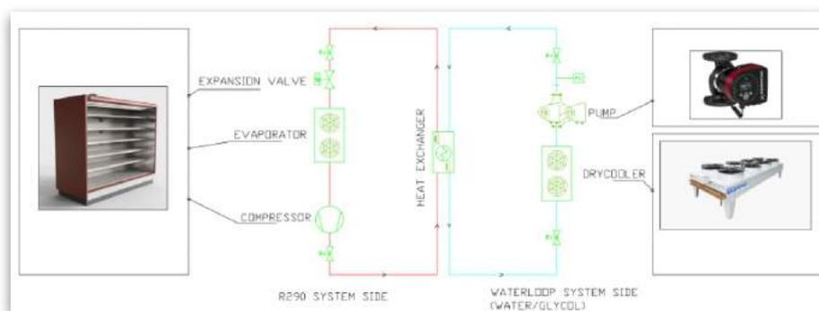
Basic diagram for the R290 water loop system
